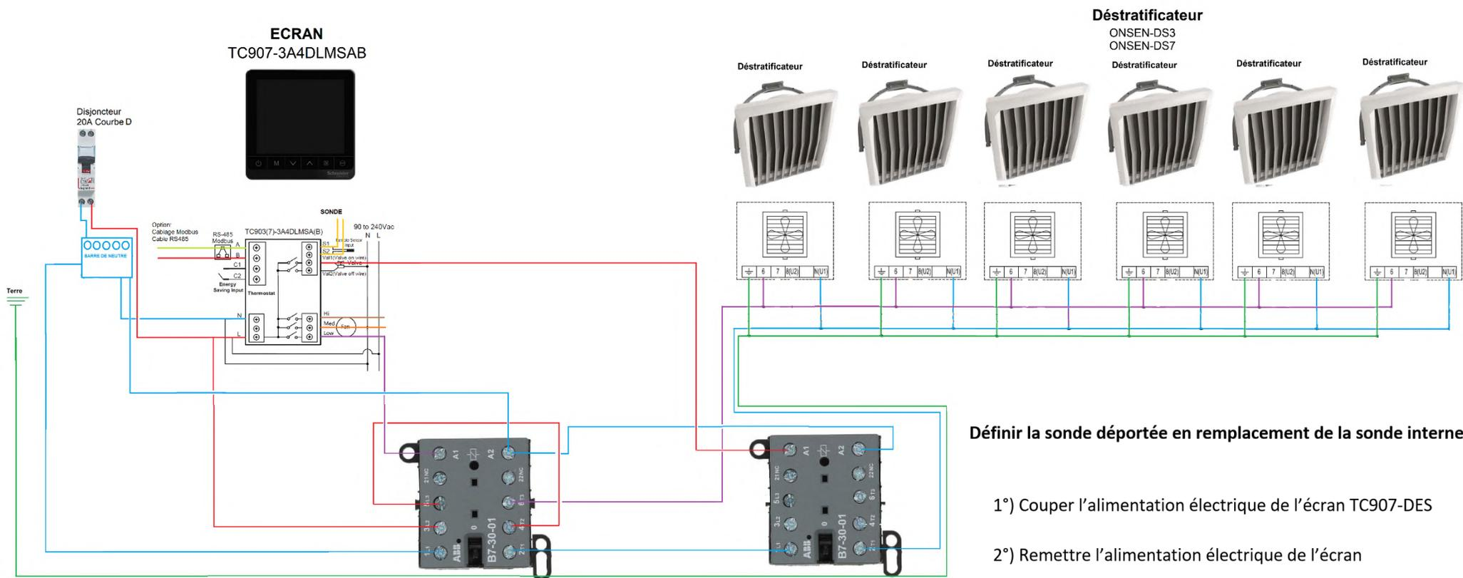
**VERSION AVEC RELAIS POUR RACCORDEMENT 6 DESTRAFIFICATEURS SUR 1 ECRAN TC907**
