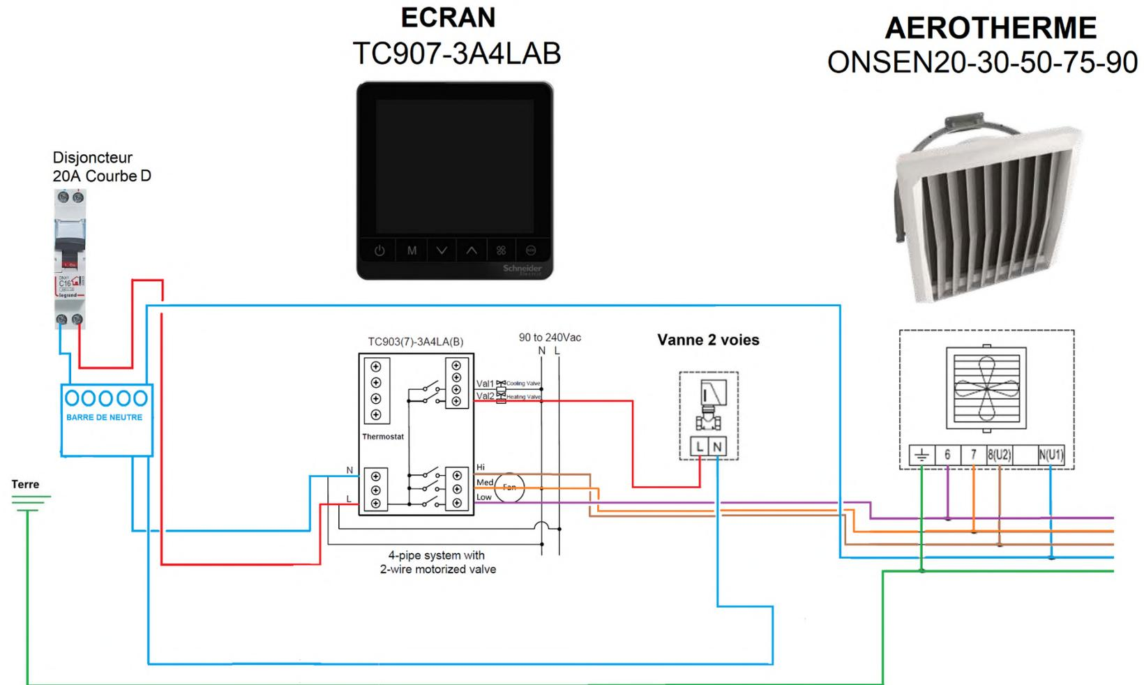
**VERSION AVEC RELAIS POUR RACCORDEMENT 6 AEROTHERMES SUR 1 ECRAN TC907 CABLAGE DES 3 VITESSES**
